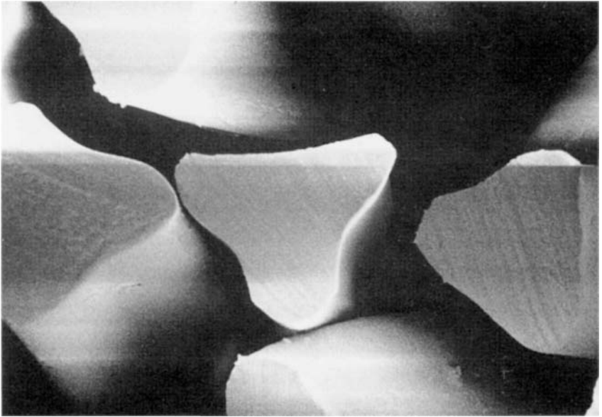
3.2 Cross-section of trilobal nylon fibres \times 1000 .
